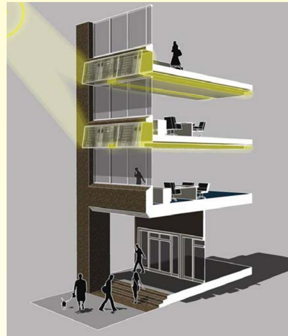
This schematic shows how the solar canopy array captures the sunlight and moves it into the interior of a building for use.
